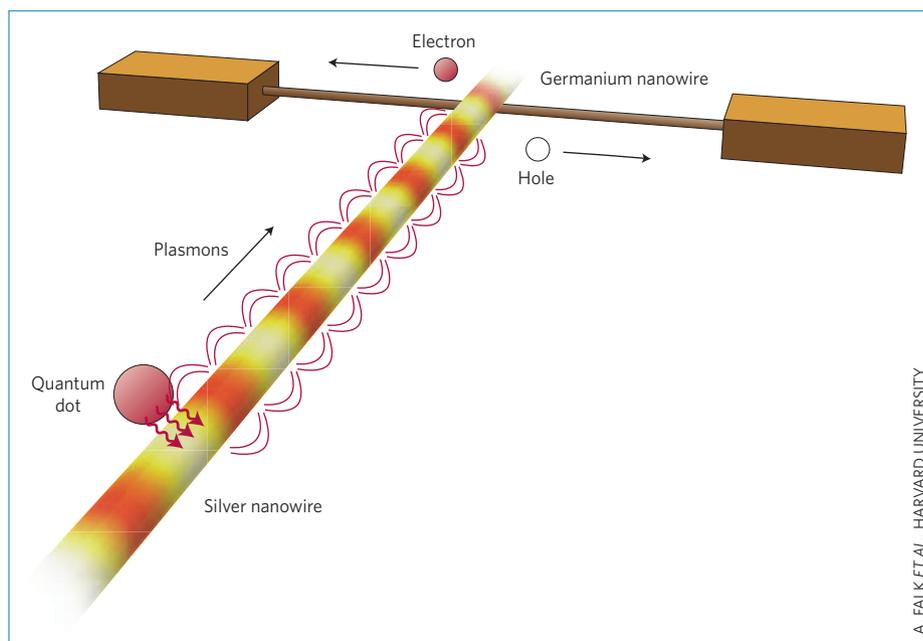
**Figure 1** | Schematic representation of a Ag nanowire, acting as a launching pad for SPs and a crossing Ge nanowire, which supports an electrical current whenever electron–hole pairs are excited by the SP electric field at the Ag–Ge contact. In the scheme, SPs are created by the de-excitation of a QD.
