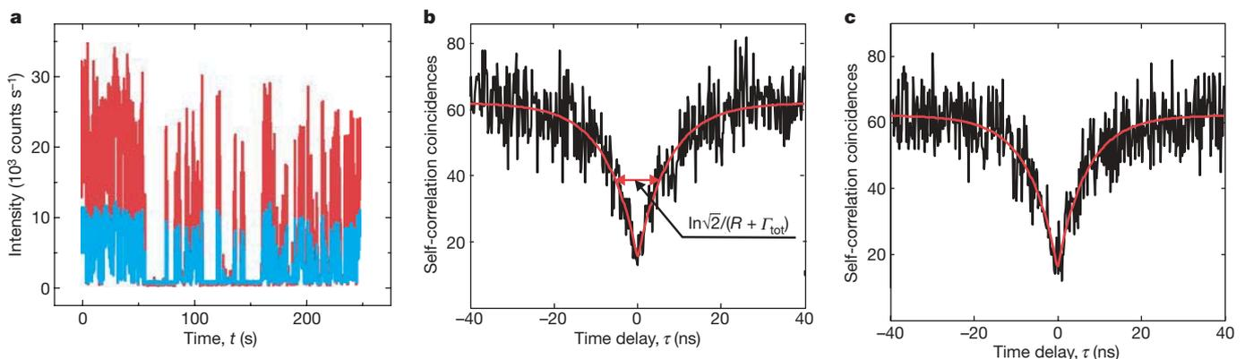
**Figure 3 | Demonstration of single surface plasmon generation.** **a**, Time trace of fluorescence counts (red curve) from a coupled quantum dot and scattered light (blue) from the end of the coupled nanowire. Fluctuations are due to quantum dot blinking<sup>19</sup>. **b**, Second-order correlation function  $G^{(2)}(\tau)$  of quantum dot fluorescence. The number of coincidences at  $\tau = 0$  goes almost to zero, confirming that the quantum dot is a single-photon source.
