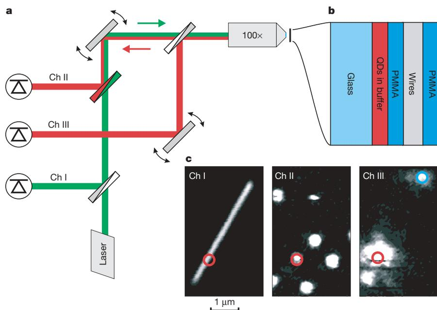
**Figure 2 | Experimental set-up.** **a**, Three-channel confocal microscope with 532 nm laser excitation source. **b**, Layout of sample containing quantum dots and nanowires. **c**, Left, channel I: nanowire image. Middle, channel II: image of quantum dots. The red circle denotes the position of the coupled quantum dot, and the same point is also denoted in the leftmost image.
