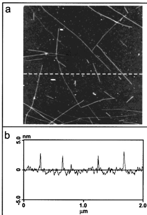
**Figure 4.** (a) AFM image of SWNTs grown from 3 nm average diameter catalyst on an oxidized silicon surface. The image is  $2\ \mu\text{m} \times 2\ \mu\text{m}$ . (b) Height cross-section taken along the white dashed line in (a). The diameters of nanotubes in the cross-section are (from the left) 2.86, 2.55, 2.56, and 3.11 nm, respectively.
