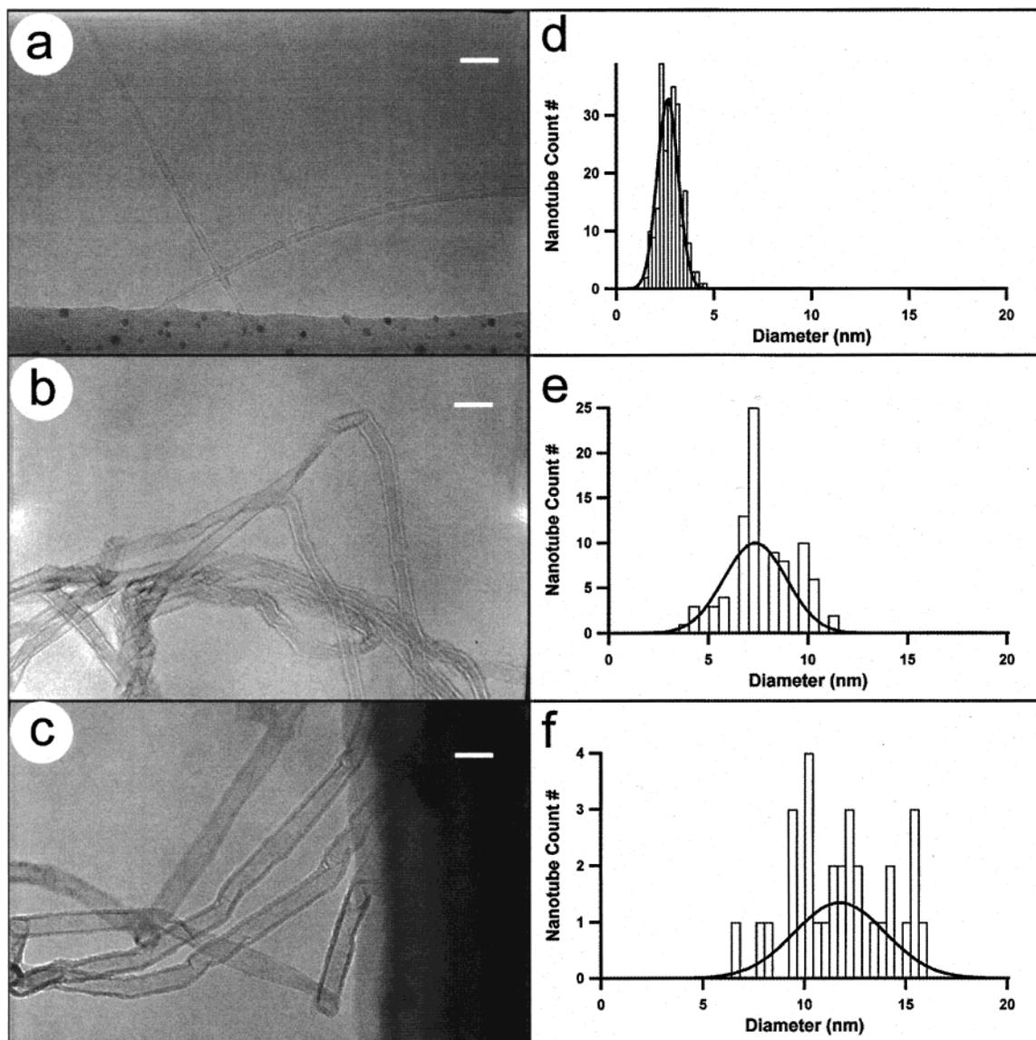
**Figure 3.** TEM images of carbon nanotubes grown using (a) 3, (b) 9, and (c) 13 nm average diameters iron nanoclusters. Scale bars are 20 nm for (a), (b), and (c). Corresponding histograms of the nanotube diameters are plotted in (d), (e), and (f), respectively. The solid lines correspond to Gaussian fits.
