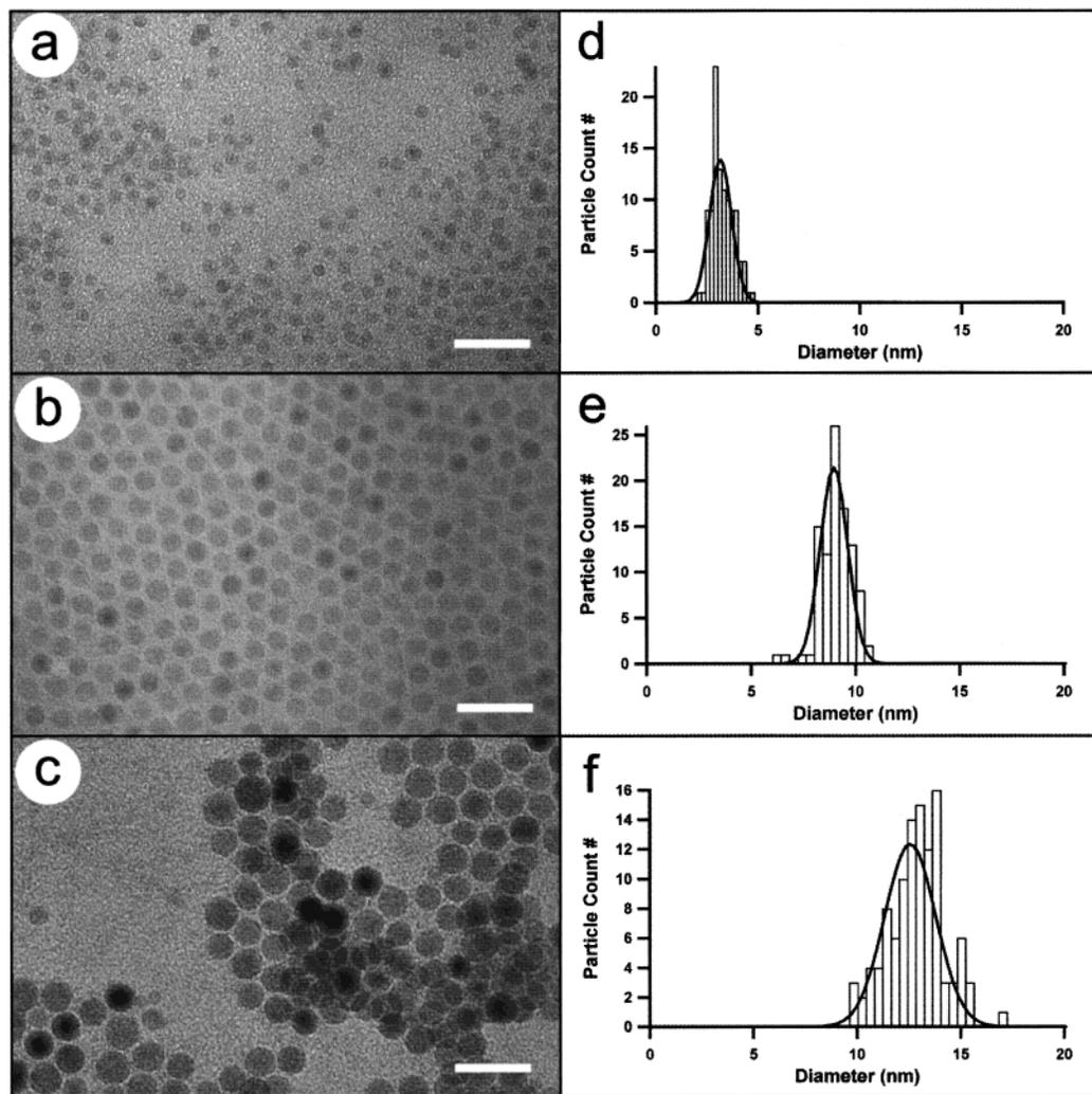
**Figure 2.** TEM images of iron nanoclusters produced by solution-phase synthesis using (a) oleic acid, (b) lauric acid, and (c) octanoic acid. The scale bars are 30 nm. Corresponding histograms of the nanocluster diameters are plotted in (d), (e), and (f), respectively. The solid lines correspond to Gaussian fits.
