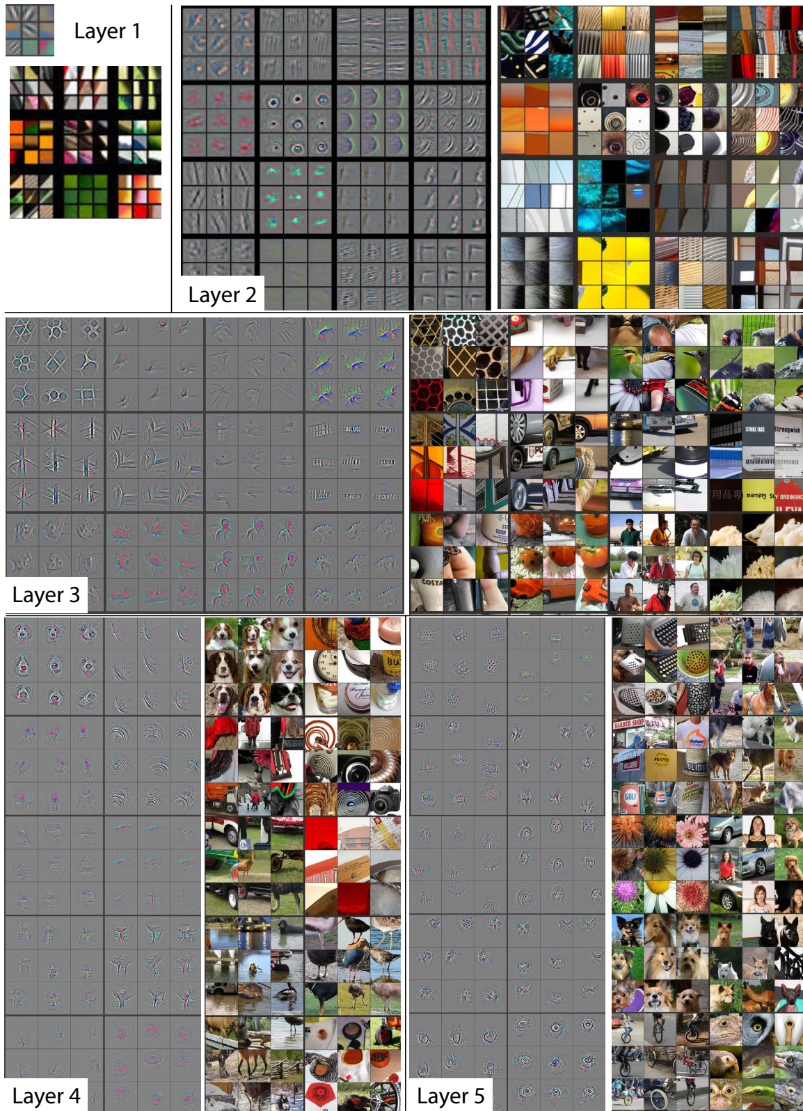
Figure 2. Visualization of features in a fully trained model. For layers 2-5 we show the top 9 activations in a random subset of feature maps across the validation data, projected down to pixel space using our deconvolutional network approach. Our reconstructions are not samples from the model: they are reconstructed patterns from the validation set that cause high activations in a given feature map. For each feature map we also show the corresponding image patches. Note: (i) the strong grouping within each feature map, (ii) greater invariance at higher layers and (iii) exaggeration of discriminative parts of the image, e.g. eyes and noses of dogs (layer 4, row 1, cols 1). Best viewed in electronic form.
