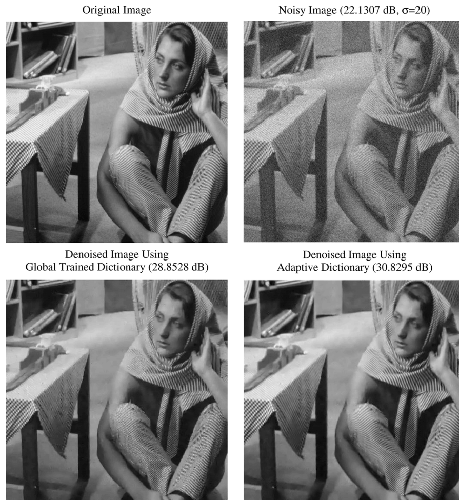
Fig. 6. Example of the denoising results for the image “Barbara” with \sigma = 20 —the original, the noisy, and two restoration results.
