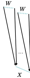
Figure 21.1: A sensor counts the photons that pass through X from incoming directions within the wedge W . This gives us \Phi(W, X) , a measurement called radiant flux.
