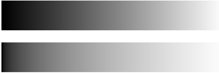
Figure 19.5: The data in the top image is a linear ramp of colors, thus displaying (on a monitor) equally spaced bins in [R', G', B']^t coordinates. In the lower image, a linear ramp has been gamma corrected before being stored. Thus, displaying (on a monitor) equally spaced bins in [R, G, B]^t coordinates. This should appear to move quickly out of the dark regime, and spend more buckets on bright values.
