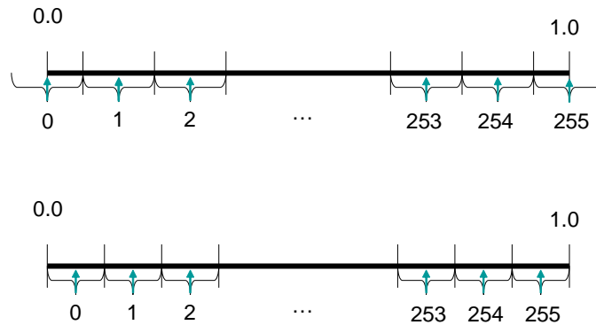
Figure 19.6: Two different mappings between real and byte values. Going from real to byte, we quantize each real range to the shown integer value. Going from byte to real we use the small cyan arrows.
