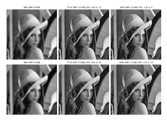
Fig. 3.3. Recovered results from FTVd and ADM. In both rows from left to right: blurry and noisy image (B&N), results recovered by FTVd and ADM, respectively. CPU and It. represent running time and iteration numbers, respectively. Top row:  $std=10^{-2}$ ; Bottom row:  $std=10^{-3}$ .
