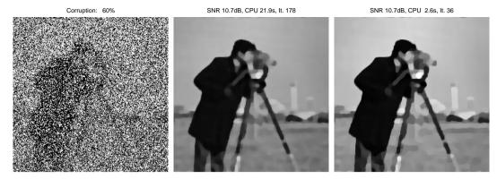
Fig. 4.2. Grayscale image results of FTVd and ADM on  $TV/L^1$ . Left: blurry and noisy image (blurred by average kernel with hsize=9 and corrupted by 60% salt-and-pepper noise); Middle: recovered by FTVd; Right: recovered by ADM.
