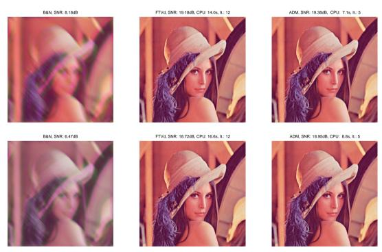
Fig. 4.1. RGB image results from FTVd and ADM. In both rows from left to right: blurry and noisy image (B&N), results recovered by FTVd and ADM, respectively. Top row: results recovered from within channel blurring; Bottom row: results recovered from cross-channel blurring.
