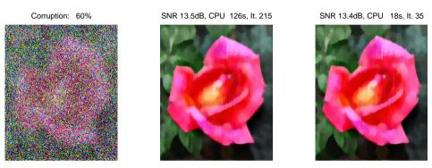
Fig. 4.3. RGB image results of FTVd and ADM on  $TV/L^1$  problem. Left: blurry and noisy image (blurred by the same cross-channel kernel as used in Section 4.1 and corrupted by 60% salt-and-pepper noise); Middle: recovered by FTVd; Right: recovered by ADM.
