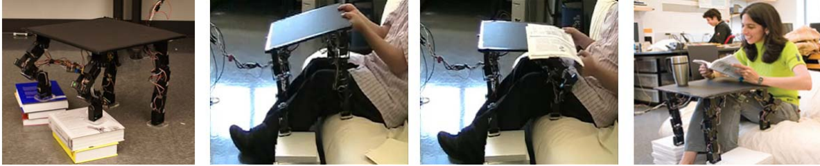
Figure 1: The self-balancing table. The table legs are formed by modules that are programmed to jointly maintain the table surface level.
